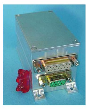
The micromax Sensor Interface is designed to complete small jobs with a microcontrollers help. Depending on the application, it can be arranged with different sensor interfaces (e.g. thermocouple amplifier, NTC amplifier). The sensordata can be processed in the microcontroller. The raw data can be filtered, linearized and sent to further CAN knots within the CAN bus interface. CANAerospace is supported.
